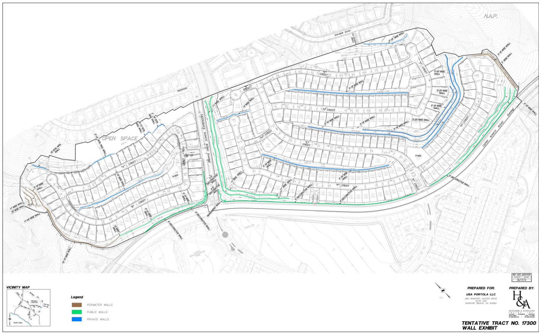
Exhibit 3-6 Portola Center North Retaining Walls
